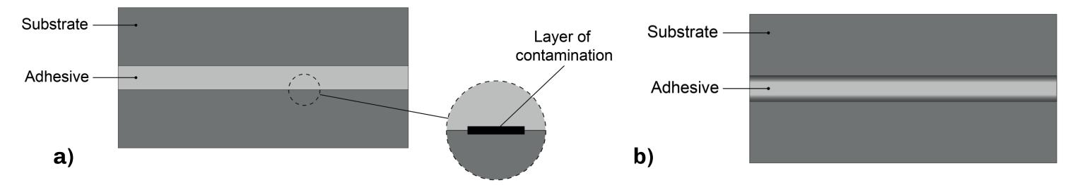
Figure 1 – Contamination and the adhesive/substrate interface a) and contamination absorbed by the adhesive at the interphase b).
