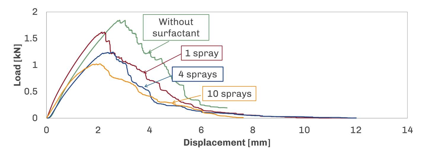
Figure 3 - Representative load-displacement curves for DCB tests for each contamination level
