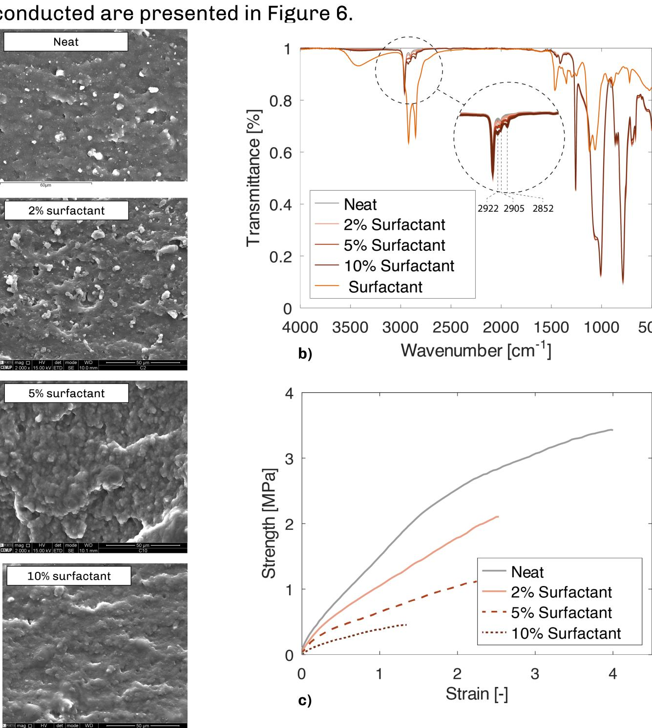
Figure 6 – SEM analysis a), FTIR analysis of the fracture surface b) and bulk tensile test results c).
