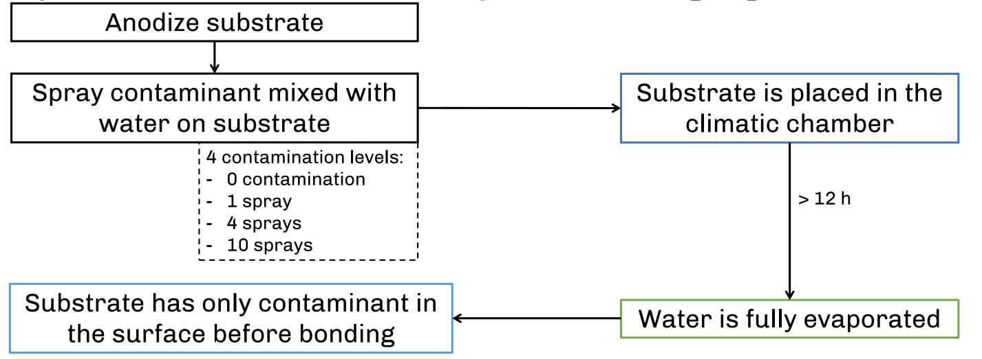
Figure 2 – Substrate treatment procedure prior to bonding.
