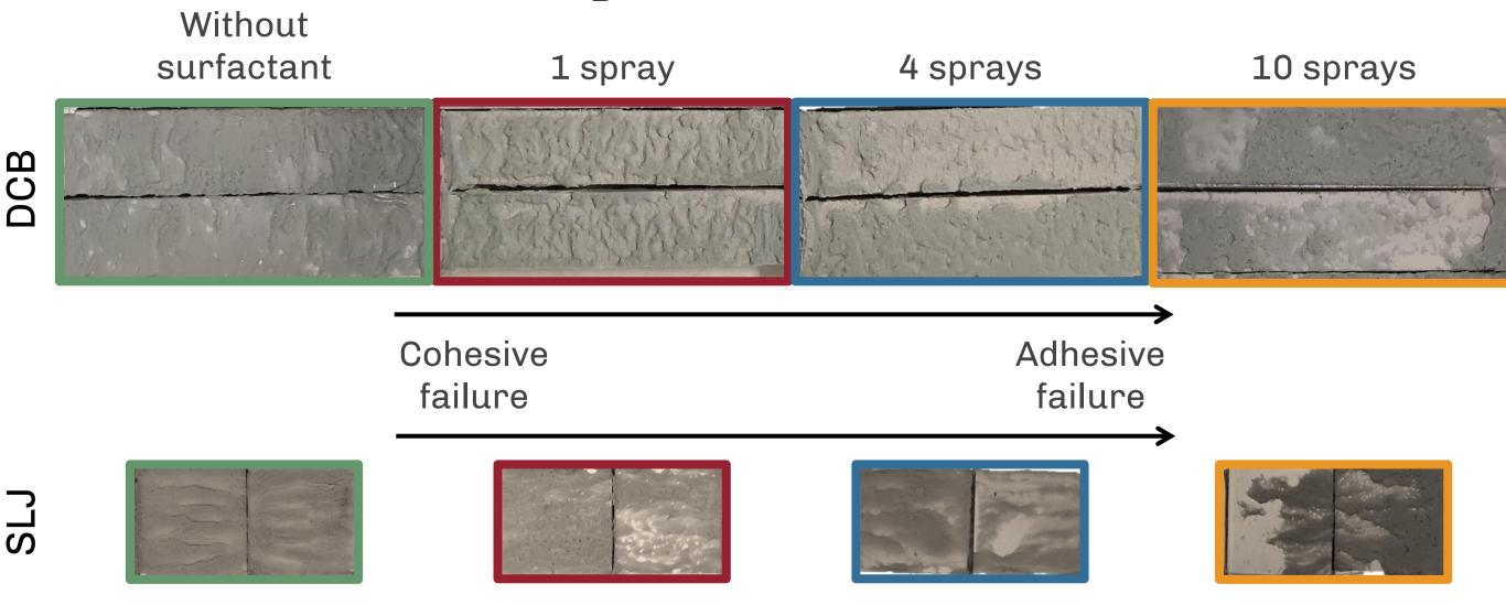
Figure 5 - Fracture surfaces for each contaminant level tested, for SLJ and DCB.
