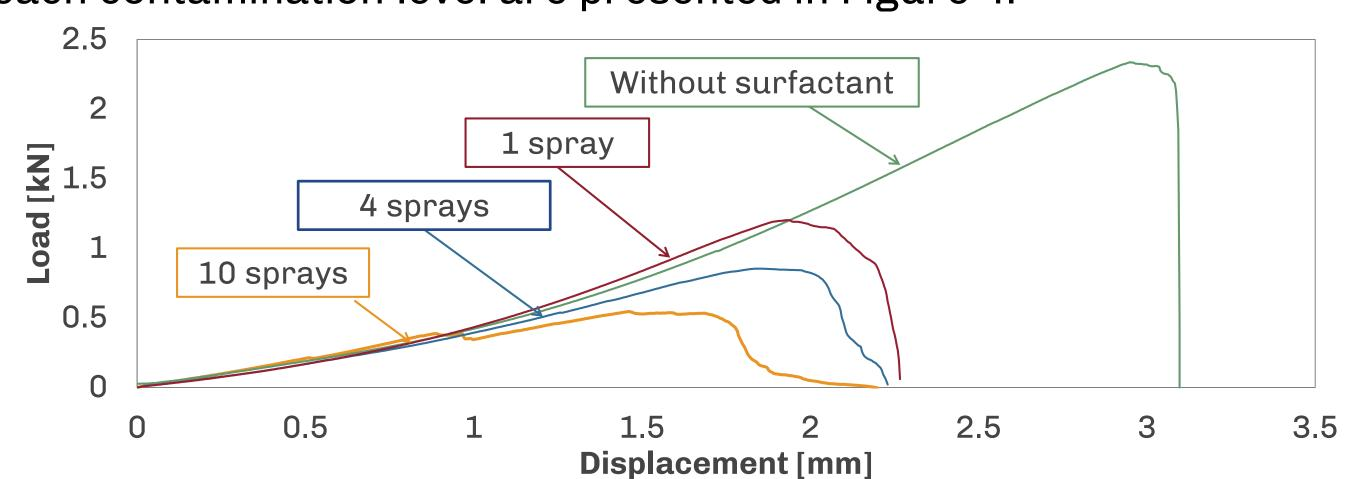
Figure 4 - Representative load-displacement curves for SLJ tests for each contamination level
